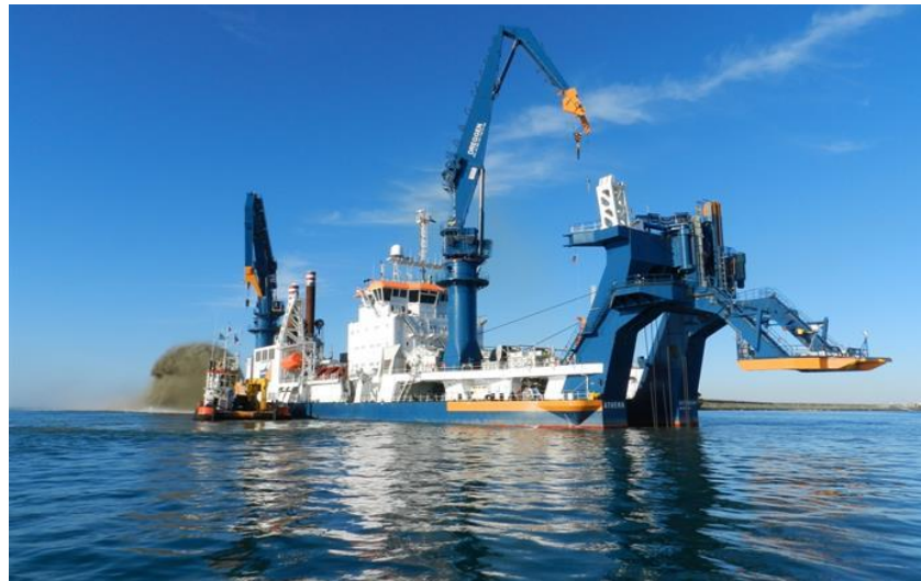
Self-propelled cutter suction dredger Athena
